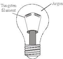
When electricity is passed through the tungsten filament it gets very hot and gives out light.
