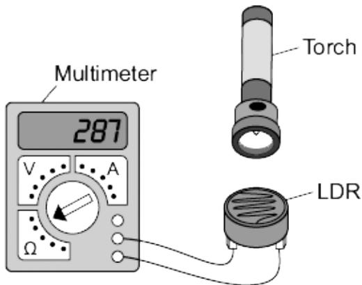
The resistance of the LDR was measured directly using a multimeter.
