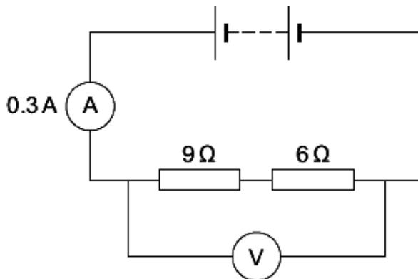
(i) Calculate the total resistance of the two resistors in the circuit.
