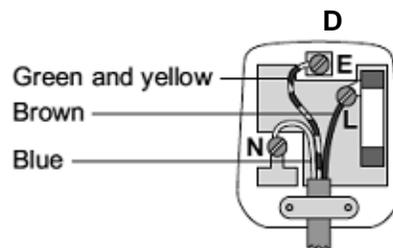
The plug that is correctly wired is
