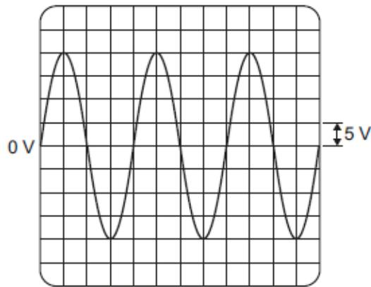
One vertical division on the oscilloscope screen represents 5 volts.
