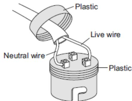
The light fitting does **not** have an earth wire connected.
