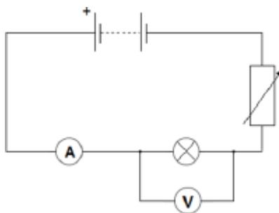
*battery in series with bulb and ammeter*
